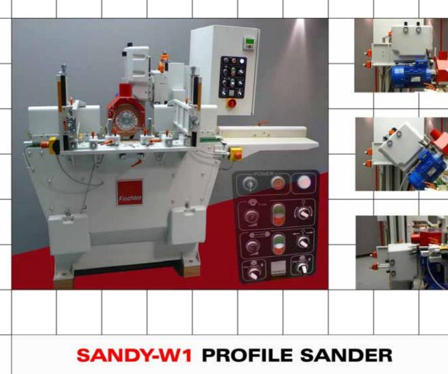
The very latest profile sander design. It is fitted as standard with a compensating cylinder which ensures that the sanding disc applies uniform pressure to the strip even if the material is slightly warped. The pressure can be adjusted individually.
